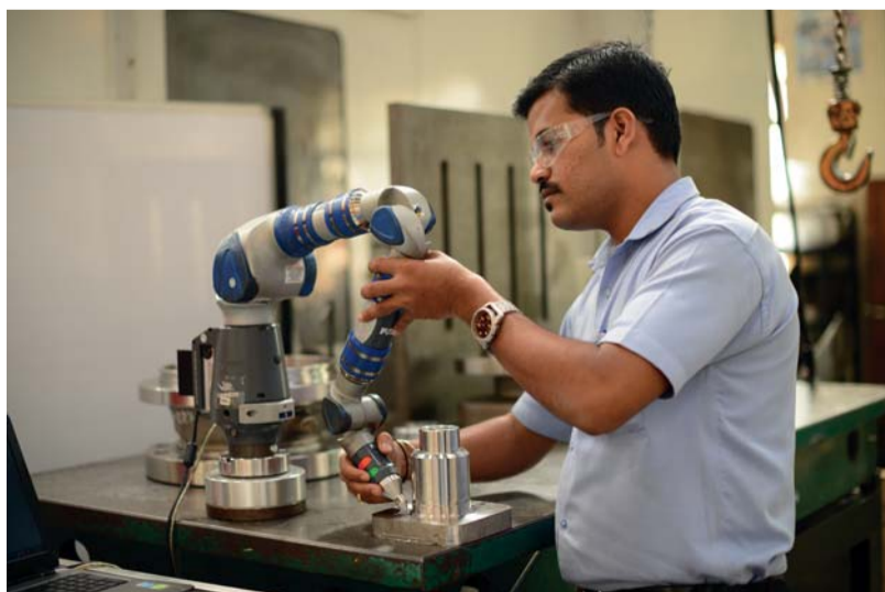
An employee uses a FARO measuring device, one of many tools used to ensure valve quality.
